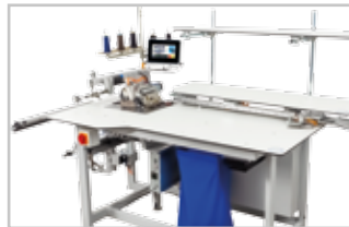
Ekrandan her iki uç noktaya mola ayarı yapabileme Ability to adjust the stitch sewing from the screen to both endpoints
