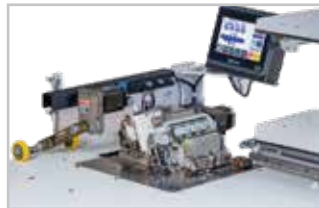
Ekrandan her iki uç noktaya mola ayarı yapabilmek Ability to adjust the stitch sewing from the screen to both endpoints
