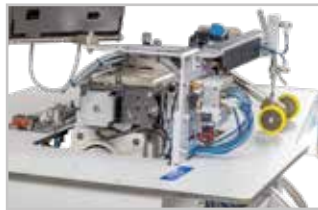
Ekrandan her iki uç noktaya mola ayarı yapabilme Ability to adjust the stitch sewing from the screen to both endpoints
